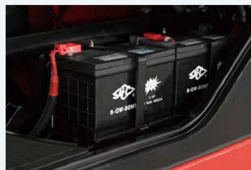
The battery is located above the fuel tank, there's battery box and adiabatic plate between them to prolong the battery's working life.
