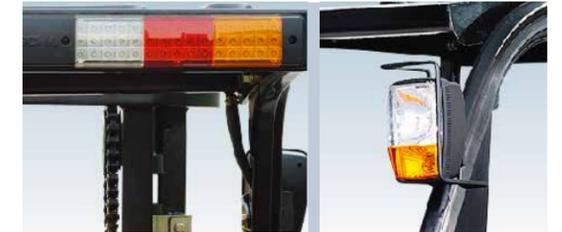
The new efficiency LED lighting system and new type reflector reduce energy consumption, improve illumination performance and prolong working life.
