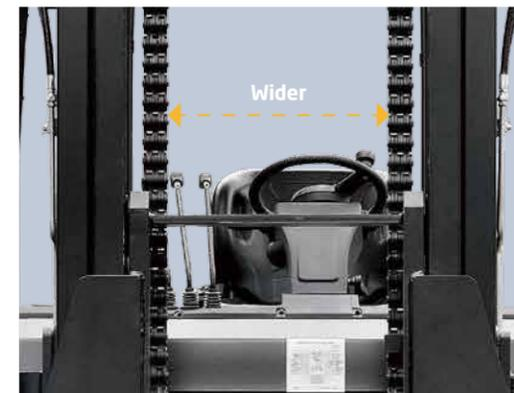
The new design mast provides broad forward visibility due to outside located hydraulic pipes of fork positioner.
