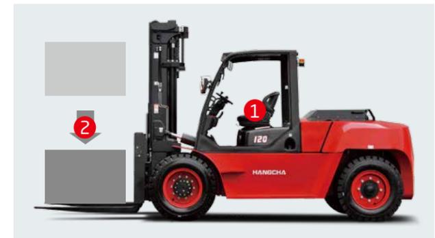
1. The seat sensor system incorporates lifting/tilting and traveling locking function. When the operator leaves the seat, the system automatically locks lifting/tilting and disables traveling to ensure safety.
