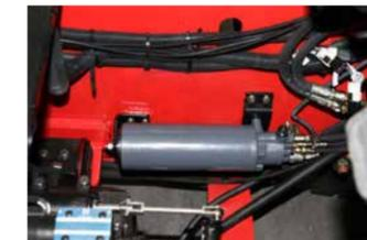
There's an energy accumulator applied in the braking system, which means when the engine is shut down, it can also provide more than 4 times emergency brake.
