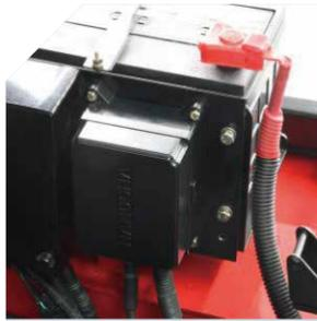
All the controllers, relays, and safety fuses are allocated in the controller box, free to water and dust. The main electronic components are waterproof, which is capable operator in severe environment.
