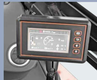
The newly designed LCD instrument has more comprehensive functions and more stable performance. It can display the important information such as truck status and engine faults... So that the operator can understand the truck status more intuitively and facilitate maintenance.
