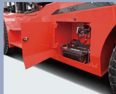
Battery compartment is easy to open for easy maintenance.
