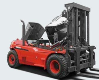
Thanks to the unique design, cab can be tilt without any tools, major service items can be reached easily by tilting the cabin, maximized access is possible.
