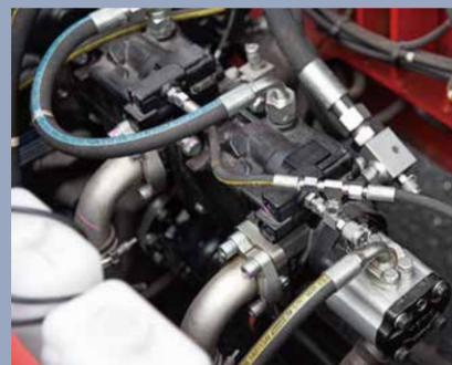
Load sensing hydraulics provide high efficiency and energy saving, reducing hydraulic oil working temperature and also extending the life of hydraulic components and seals.
