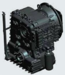
ZF gear box with micro-electronic control provides for three-shift power shifting, travelling is stable and accurate.
